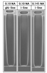
**Fig. 9:** 5µm vias in 50µm of the **p**hotoresist demonstrated using all three configurations.
